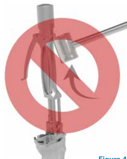
Figure 43b Do Not Hit the Tamp in Retrograde
