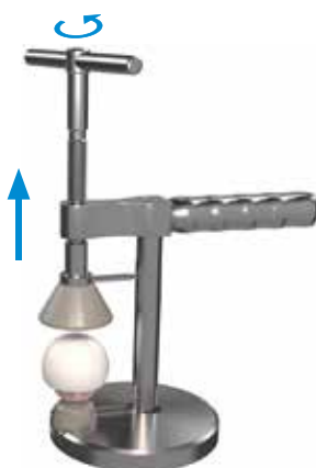
Fig. 30 Open the press completely by rotating the press Handle counterclockwise. Position and place the Liner on the head (Fig. 30).
